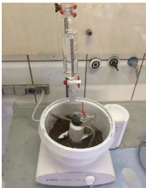
Fig. 6. Setup for dry digestion in laboratory
