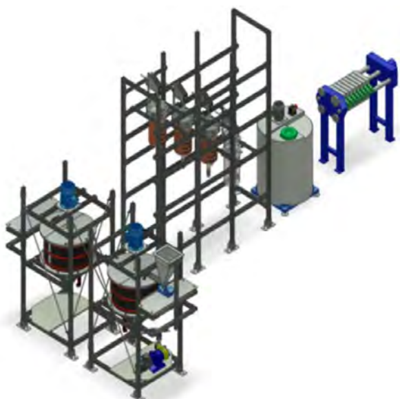
Fig. 9. Sketch of equipment for leaching, neutralisation and filtration at the pilot plant
