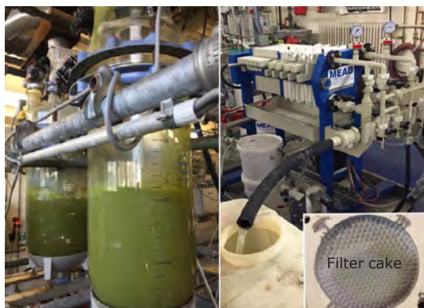
Fig. 8. Dry digestion reactors and filter press at the pilot plant
