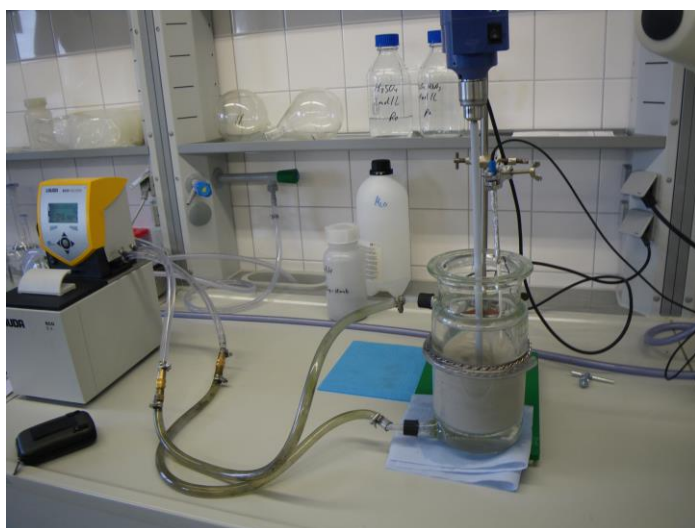
Figure 1: Leaching experiments under a) atmospheric pressure b) high pressure
