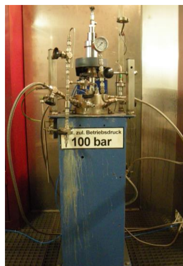
Figure 1: Leaching experiments under a) atmospheric pressure b) high pressure
