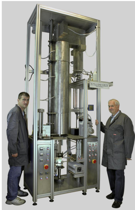
Fig. 3: Ultrasonic Spray Pyrolysis Synthesis at the RWTH Aachen University
