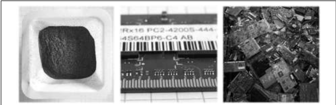
Figure 2: Samples used for experiments on TS gold leaching, from left to right: flue dust from e-waste crushing and milling processes, RAM and circuit boards
