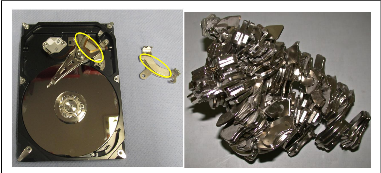
Figure 3: Hard disc drive with magnets marked (a); magnets of different hard disc drives sticking together (b)
