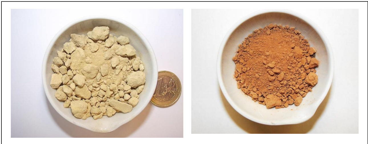
Figure 3: Ion Adsorption Clay raw material (left: Fe-hydroxide enriched material, right: hematite enriched material)
