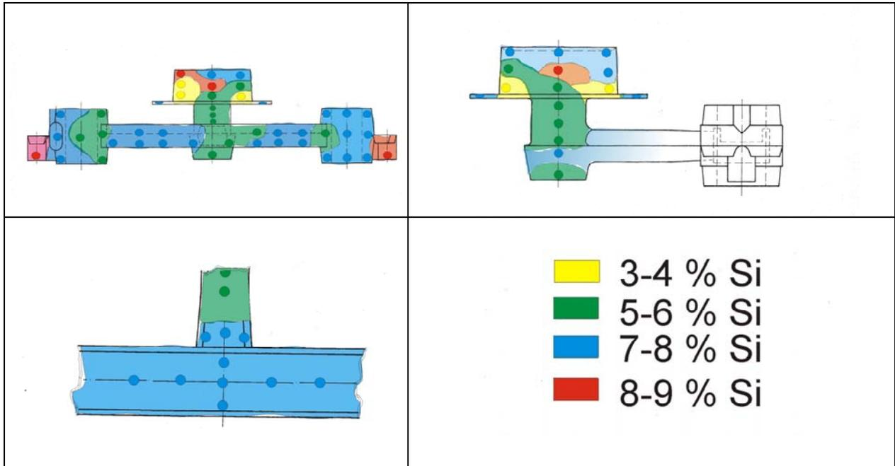
**Picture 6:** silicon content distribution of the component after step-shot tests (Spots: samples for ICP-analysis)
