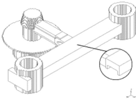
**Picture 3:** Prototype component for Thixoforming tests
