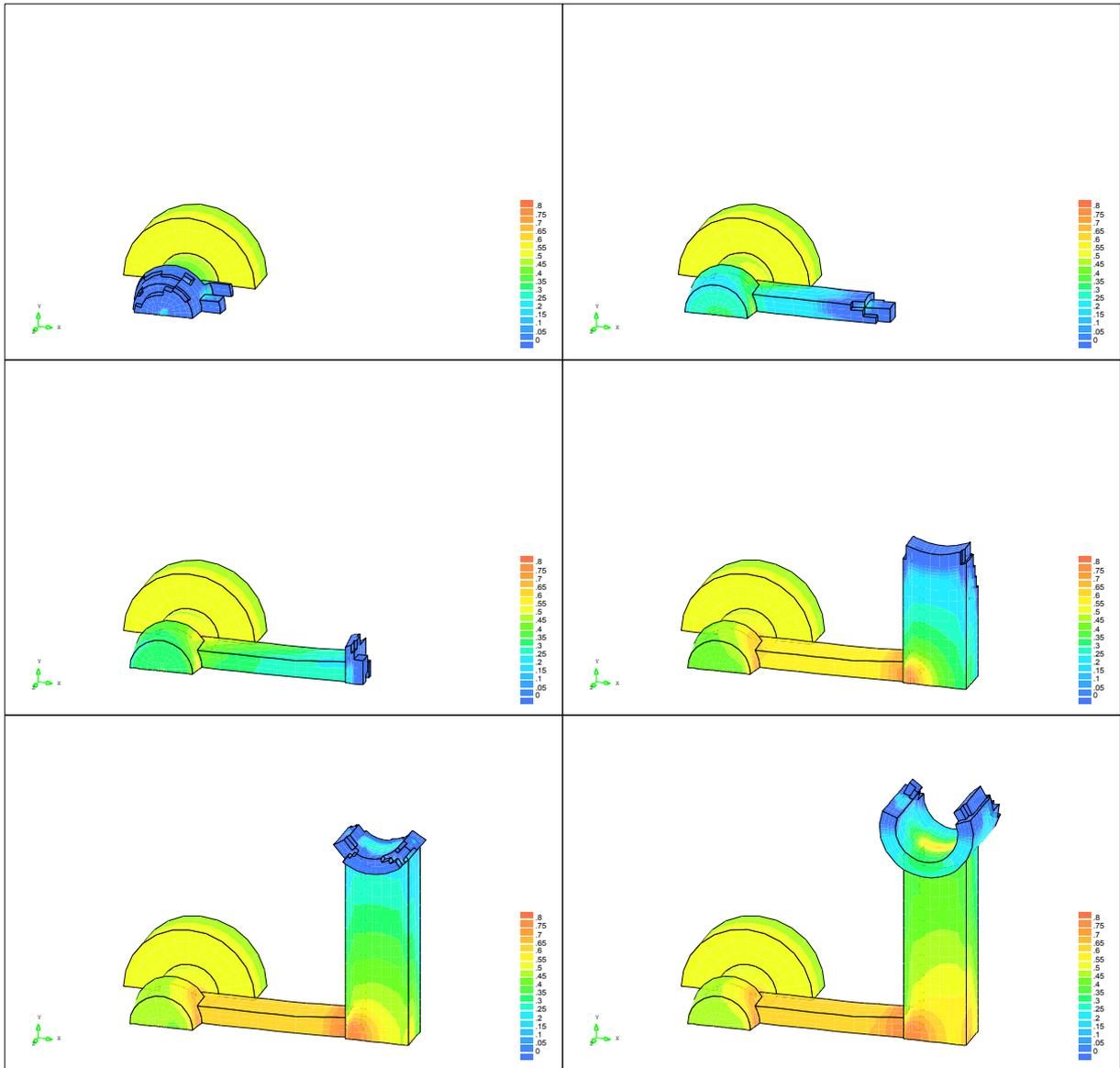
**Picture 5:** Simulation of segregation during the step shot process. Piston speed 250 mm/s.
