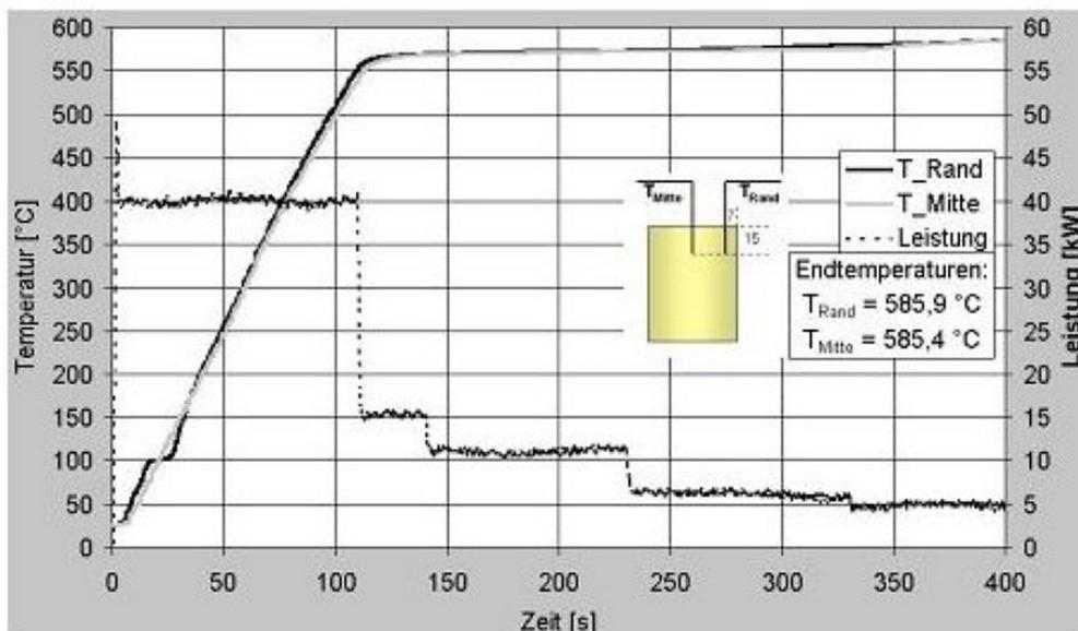
**Picture 1:** Inductive billet heating procedure (ingot material A356 (MHD); 2,2kg; dT~5 °K/s)
