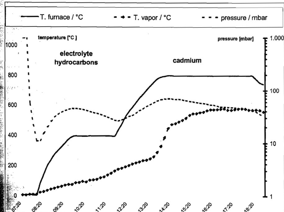
Figure 3: Temperature and Pressure while Treatment of spent NiCad-Batteries
