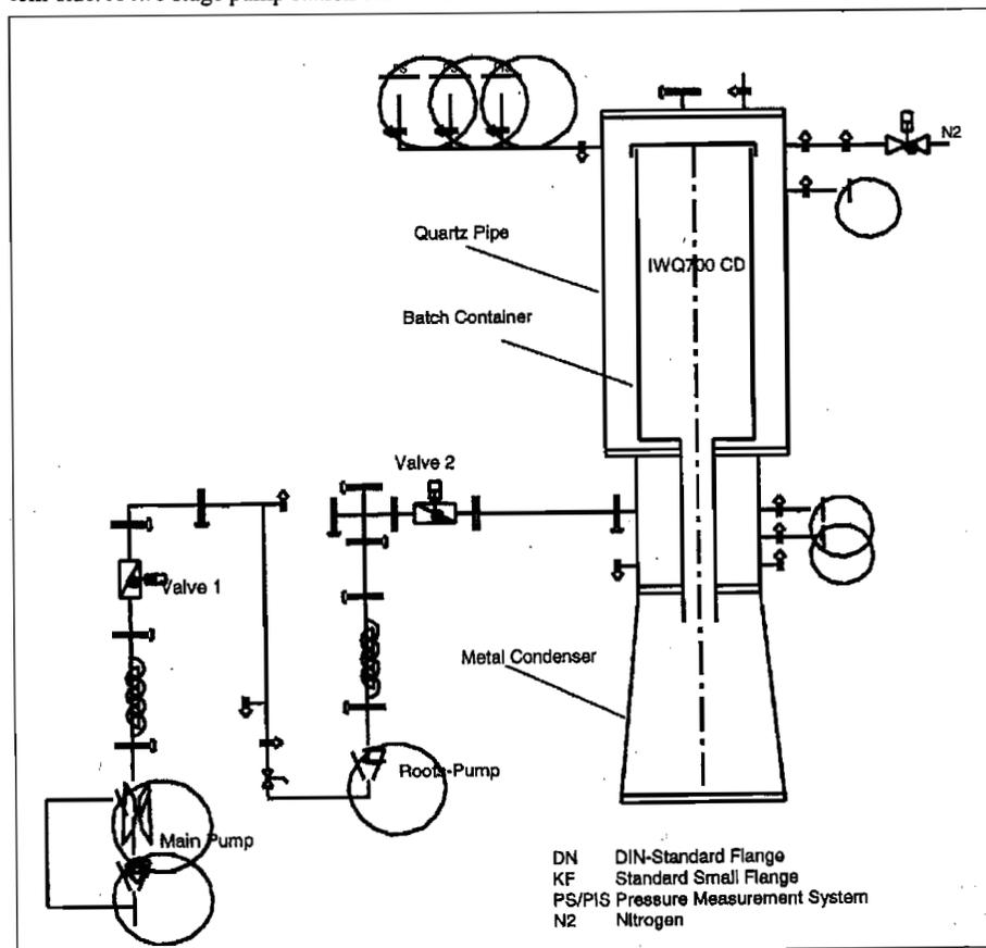
Figure 2: Schematic Design of the Vacuum-Recycling Furnace
