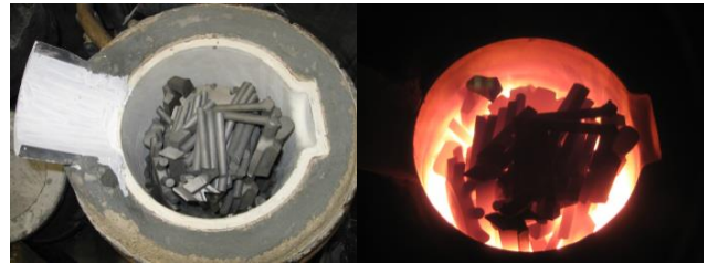
Figure 4: Vacuum induction melting of TiAl scrap
