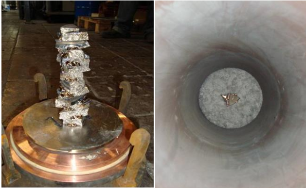
Figure 11: starting plate (left), top view of crucible with slag and starting plate (right)
