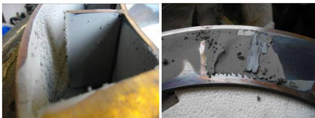
Figure 15: Powdered "metallic" material collected at the copper condenser after the experiment.
