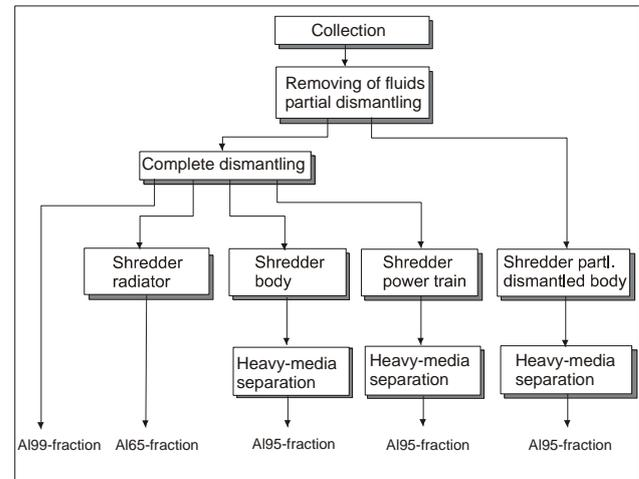
Figure 3: Recycling system of ELV in Germany
