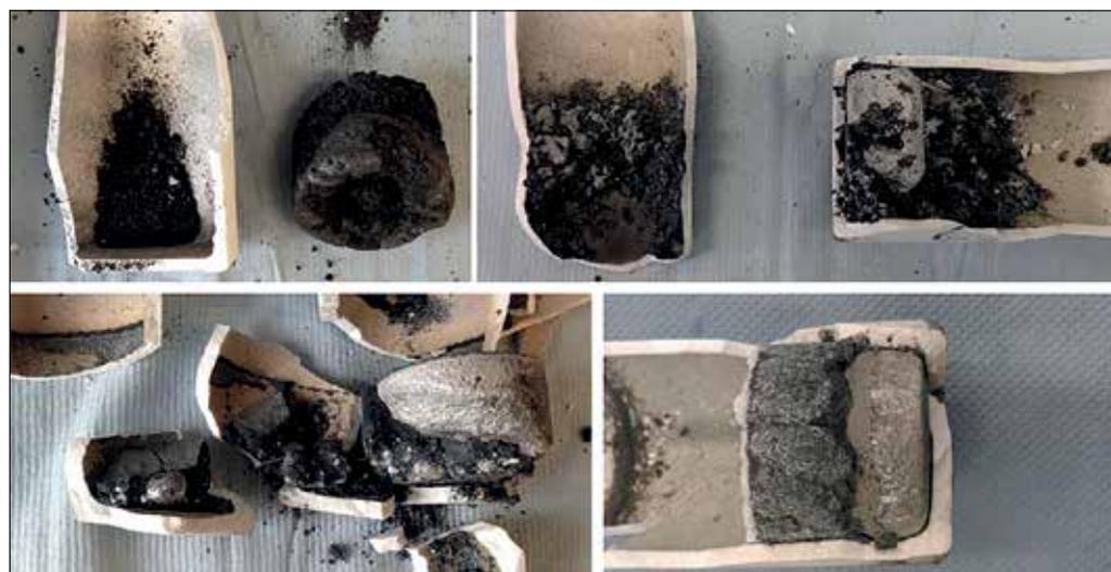
Fig. 9: Cooled samples after recycling cycles (up left: Salt/scrap = 0; up right: S/s = 1/3; bottom left: S/s = 2/3; bottom right: S/s = 1)
