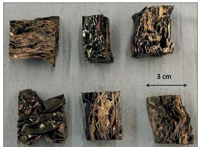
Fig. 7: Input material after pyrolysis
