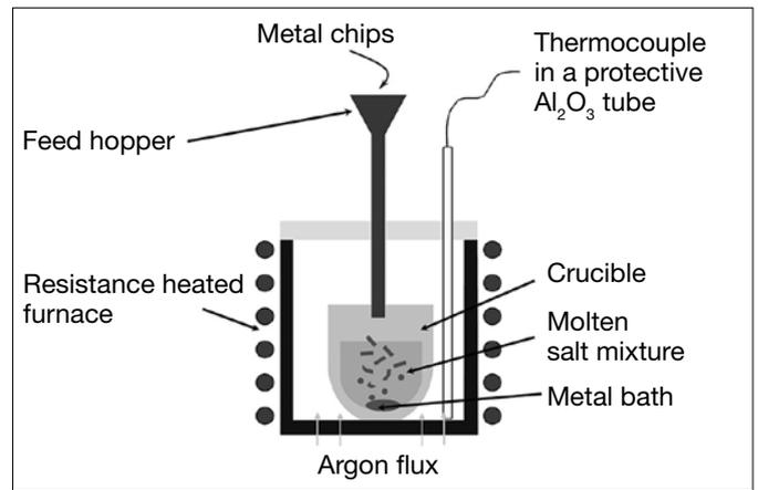
Fig. 1: Experimental set-up for the coalescence tests
