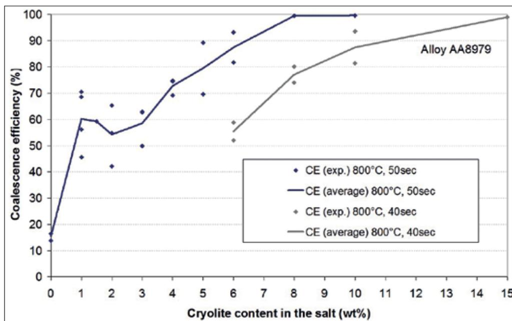
Fig. 3: Coalescence efficiency of AA 8979 (low alloyed) chips as a function of cryolite content in the salt (initial salt temperature = 800 °C)
