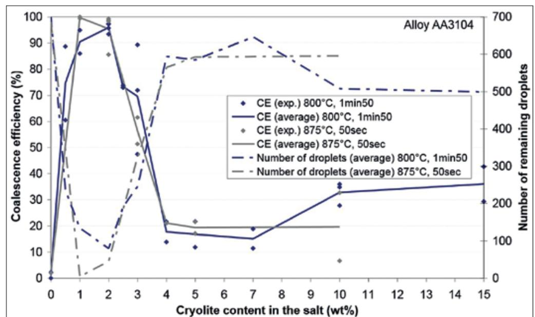
Fig. 2: Coalescence efficiency of AA3104 (0.8 to 1.3 wt.% Mg) chips as a function of cryolite content in the salt (initial salt temperature = 800 °C or 875 °C)
