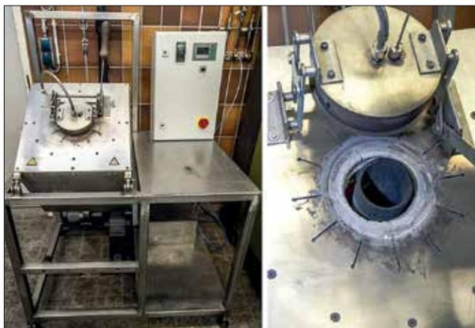
Fig. 6: Photos of the Mini TRF (left: overview, right: zoom on the opening)
