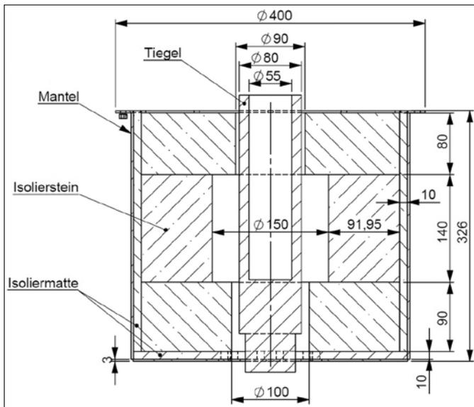
Fig. 5: Pattern of the Mini TRF (lengths in mm)
