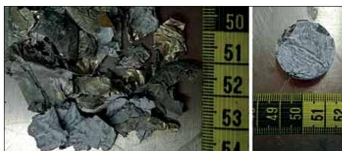
Fig. 8: Pyrolysed UBC chips at 550 °C, compact pyrolysed UBC chips
