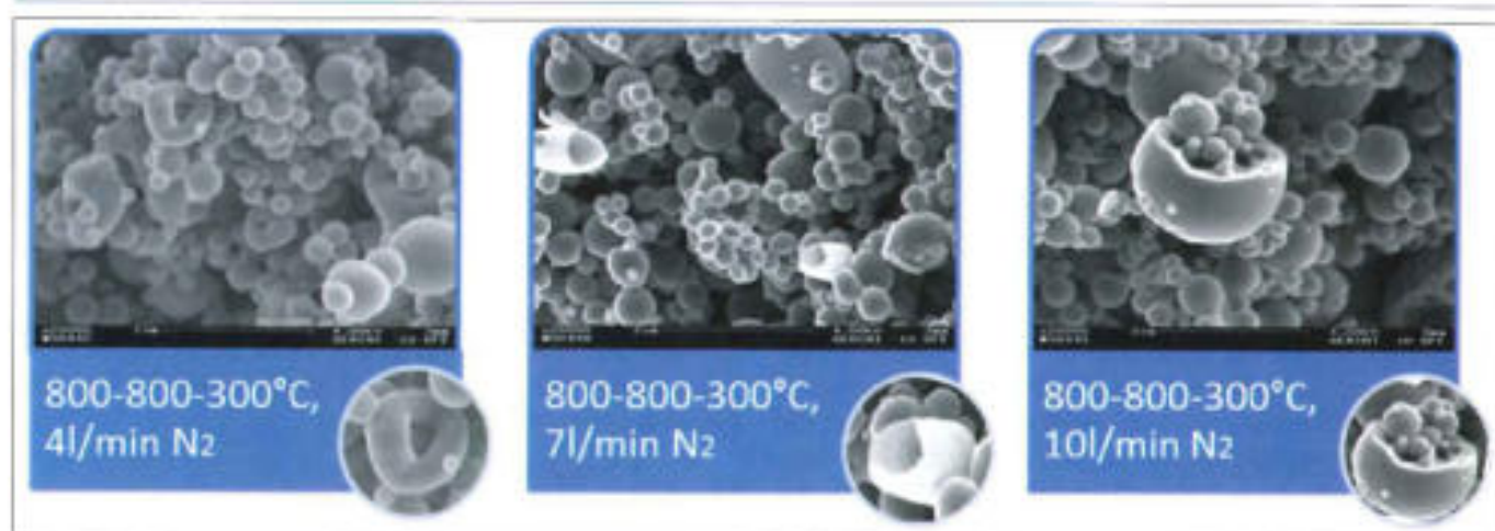
Fig. 4: SEM analysis from titanium dioxide nanopowder obtained in experiments 1 to 3 (left and right are SEM images of same experiment)
