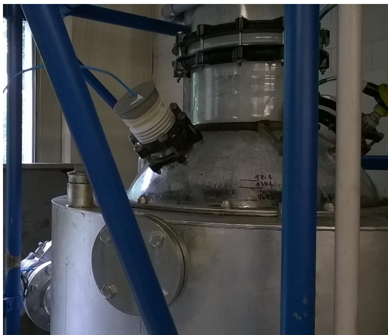
Figure 3: Leaching in 200-L reactor
