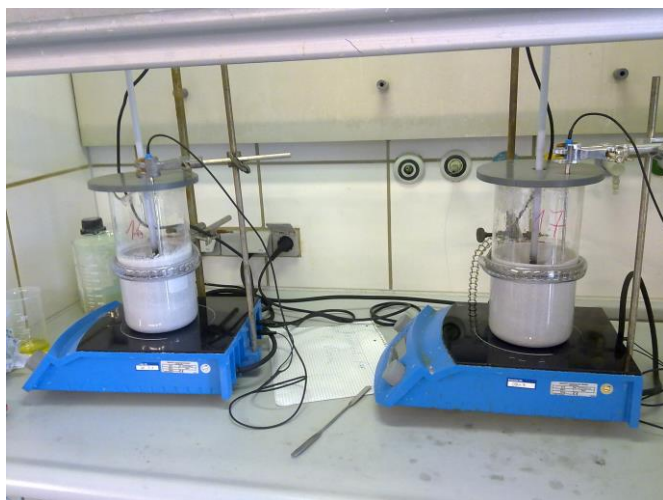
Figure 2: Leaching of a dried lead scrap in laboratory conditions
