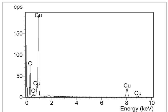
Fig. 7c: EDS analysis for copper powder obtained by reduction of CuAc using formic acid as hydrogen source
