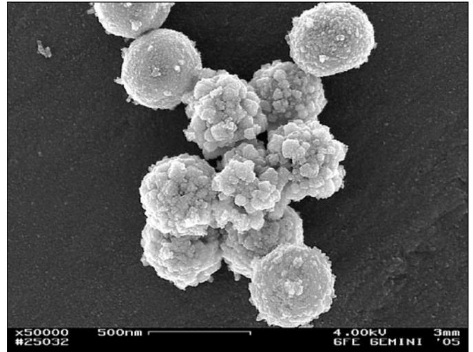
Fig. 7a: SEM micrograph of copper powder obtained at 800 °C from 0.1 mol/l CuAc (Exp. 6) by direct hydrogen gas reduction
