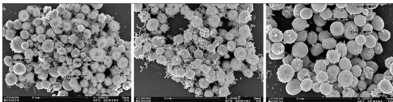
Fig. 8: SEM micrographs of hydrogen reduced Cu powder using a CuAc concentration of a) 0.05 mol/l (Exp. 8,  $1000^\circ\text{C}$ ), b) 0.1 mol/l (Exp. 7,  $1000^\circ\text{C}$ ), c) 0.2 mol/l (Exp. 9,  $1000^\circ\text{C}$ )
