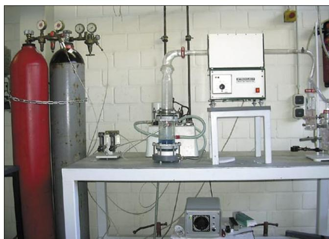
Fig. 4: Experimental apparatus for the USP-synthesis of copper particles (bottles with  $\text{H}_2$  and  $\text{N}_2$ , flowmeter, thermostat, aerosol generator, quartz tube, tube furnace, collection of powders)
