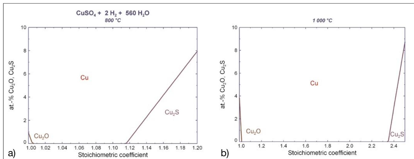
Fig. 2: Phase areas of Cu,  $\text{Cu}_2\text{O}$  and  $\text{Cu}_2\text{S}$  depending on the stoichiometric coefficient of  $\text{H}_2$  at a) 800 °C and at b) 1000 °C
