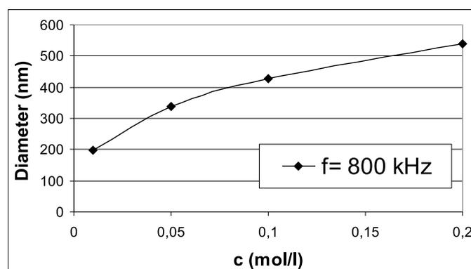
Fig. 9: Calculated particle size of copper after aerosol drying and hydrogen reduction, depending on the  $\text{CuSO}_4$  concentration in solution
