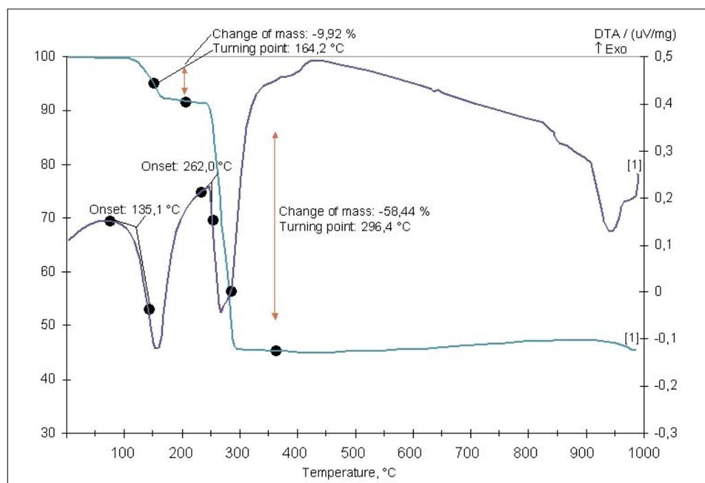
Fig. 3: DTA and TGA analysis of decomposition of copper acetate in argon
