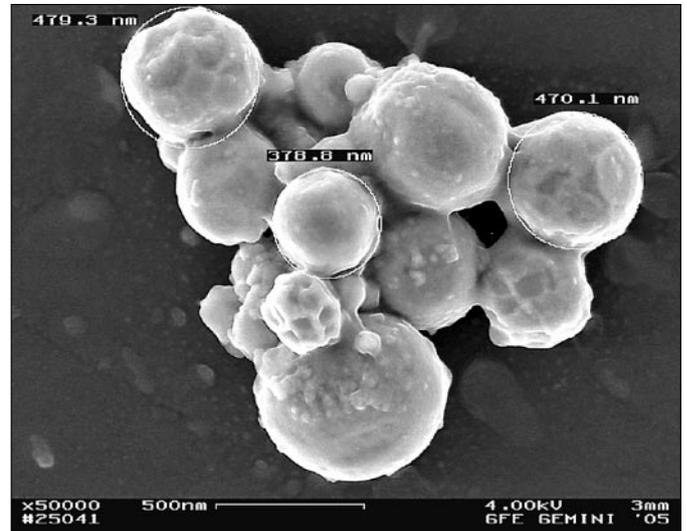
Fig. 7b: SEM micrograph of copper powder obtained at 800 °C from 0.1 mol/l CuAc (Exp. 10) by reduction using formic acid
