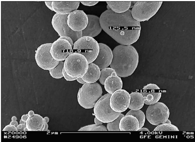
Fig. 6c: SEM micrograph of Cu powder using a  $\text{CuSO}_4$  concentration of 0.2 mol/l (Exp. 4, 1000 °C)
