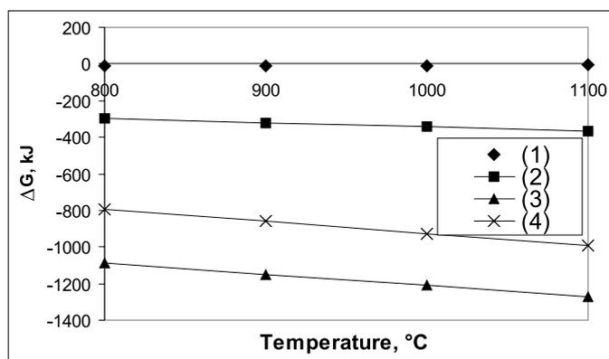
Fig. 1: Thermochemical FactSage®-analysis of hydrogen reactions with  $\text{CuSO}_4$  between 800 °C and 1100 °C
