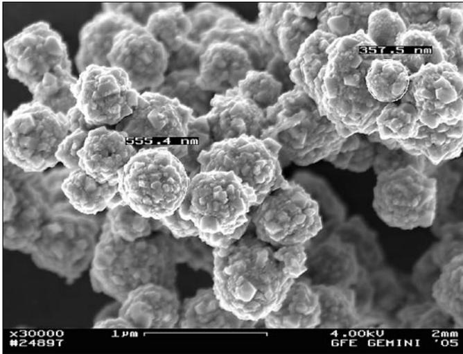
Fig. 6b: SEM micrograph of Cu powder using a  $\text{CuSO}_4$  concentration of 0.1 mol/l (Exp. 2, 1000 °C)
