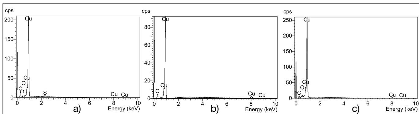
Fig. 5: a) EDS analysis for copper powder obtained in experiment (1) at 800 °C from a  $\text{CuSO}_4$  solution, b) EDS analysis for copper powder obtained in experiment (2) at 1000 °C from a  $\text{CuSO}_4$  solution, c) EDS analysis for copper powder obtained in experiment (5) at 1083 °C from a  $\text{CuSO}_4$  solution
