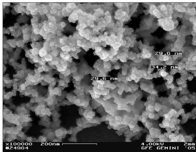
Fig. 6a: SEM micrograph of Cu powder using a  $\text{CuSO}_4$  concentration of 0.05 mol/l (Exp. 3, 1000 °C)
