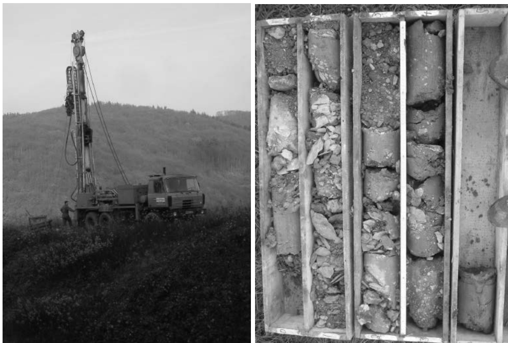
Figure 4: Picture of the drilling equipment (left) and the received drilling cores (right)
