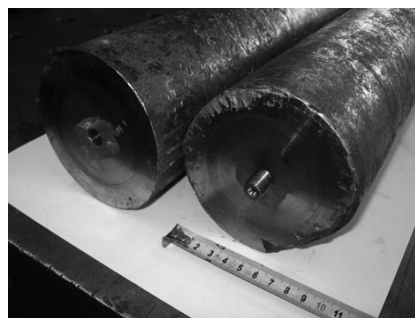
Figure 7. Mechanical bonding of two VIM ingots with a native thread rod.
