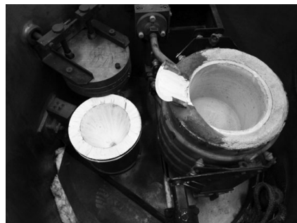
Figure 6. Vacuum induction furnace PVA VSG 100 with prepared CaO crucible. The pouring nozzle as well as the pouring cup is Y 2 O 3 coated.
