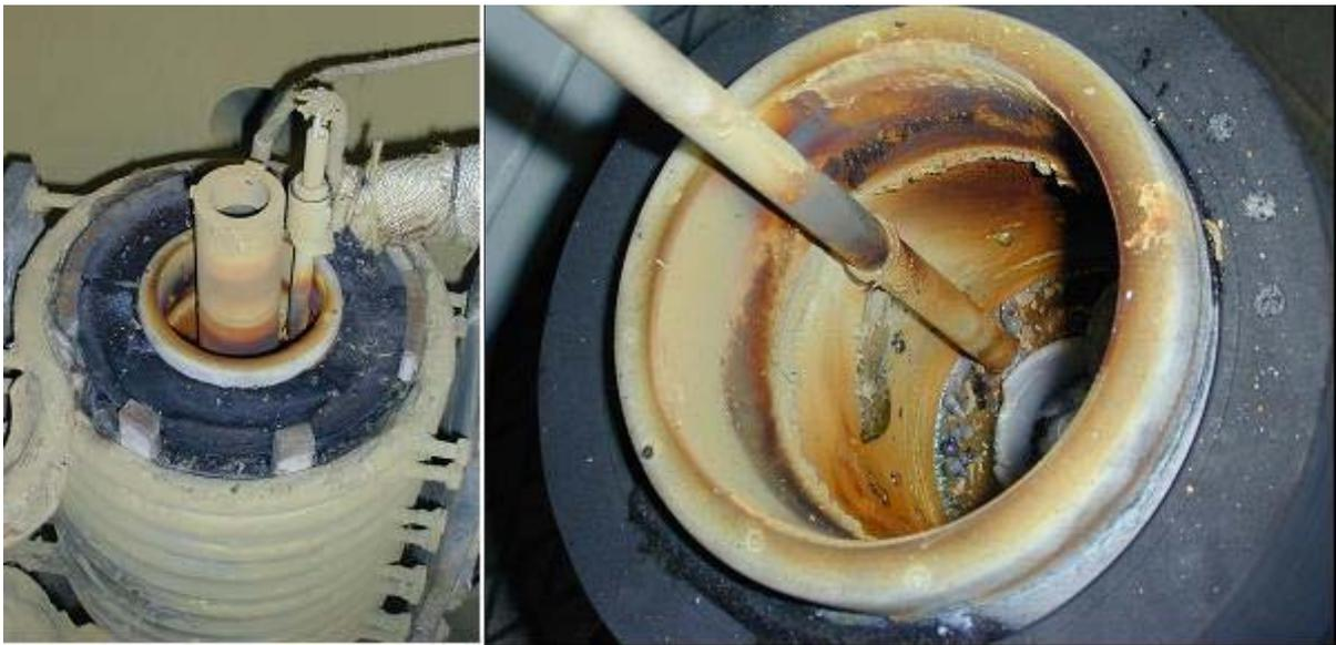
**Figure 10: Test 2. Yellow dust inside on surfaces of the crucible and the lance**
