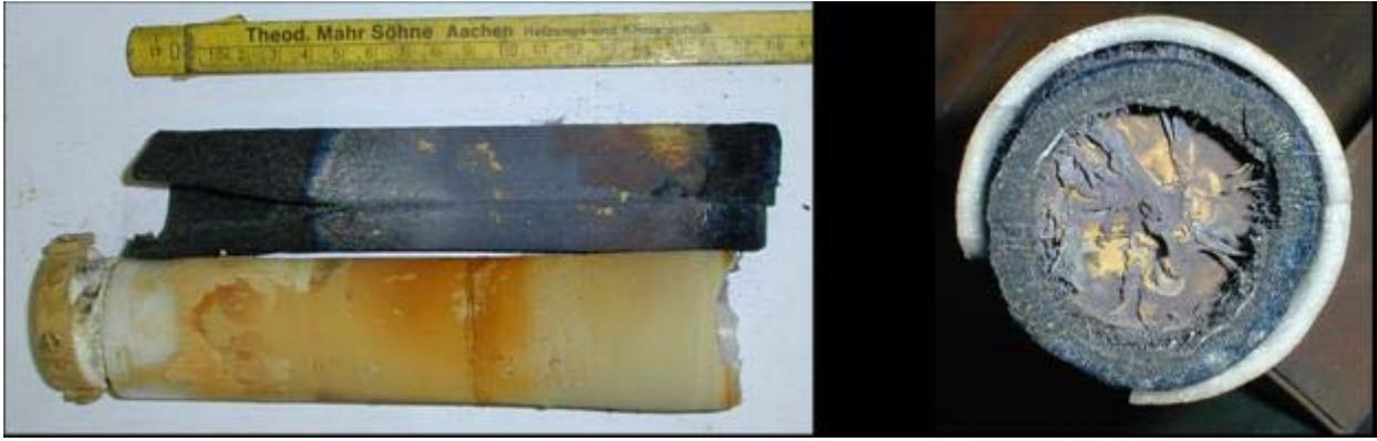
**Figure 11: Graphite felt and foil insulation converted to SiC due to plugging of the immersed silane-lance by solidified silicon metal**
