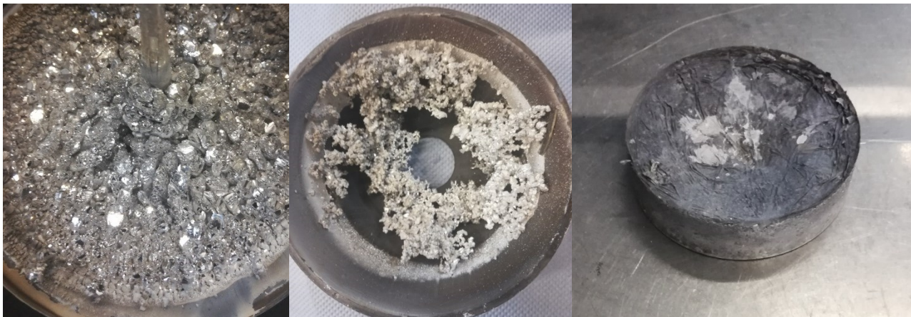
Figure 3: Condensed magnesium in the condenser (left) and in the collecting plate (middle) as well as the crucible residue (right)
