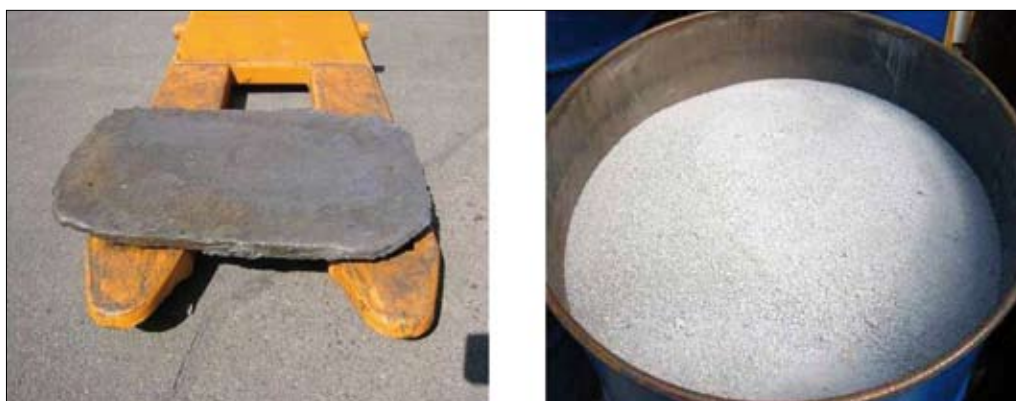
Fig. 21: Fe-Mn slab from (left) and flue dust (right) from a semi-pilot scale experiment
