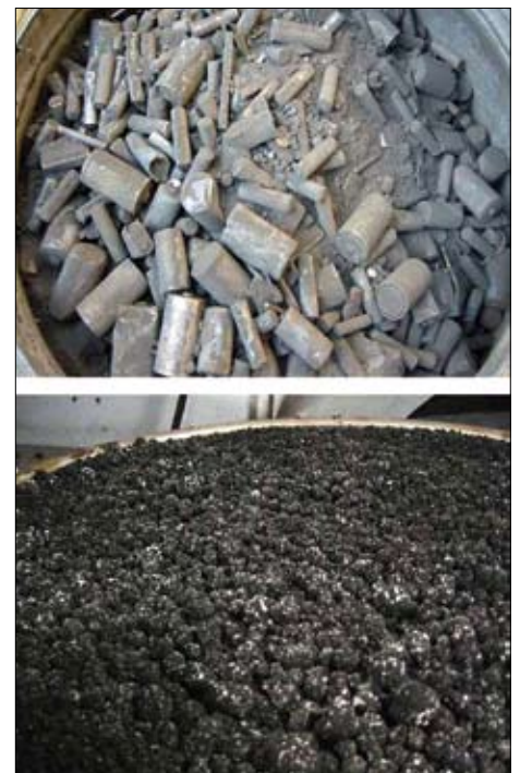
Fig. 9: Pyrolised spent primary batteries (top) and pelletised “black mass” (bottom)
