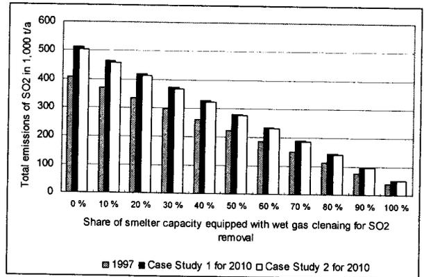
Figure 14: Total amount of SO<sub>2</sub> emitted to the atmosphere depending on the proportion of smelters operating with wet gas cleaning, assuming 2% sulphur in anodes.
