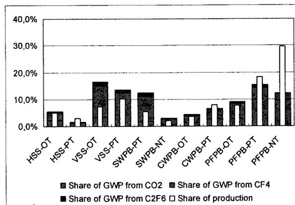
Figure 11: Share of production and emissions of CO<sub>2</sub> and CF<sub>4</sub> caused by different technical smelter categories in 2010 according to case study 1.
