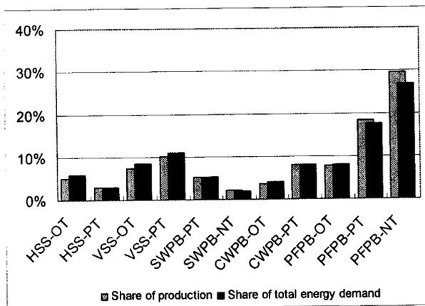
Figure 2: Share of production and total energy requirement for different technical categories of Al electrolysis cells in 2010 according to case study 1.
