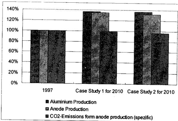
Figure 13: Comparison of aluminium production, anode production and specific CO<sub>2</sub> emissions due to anode production.
