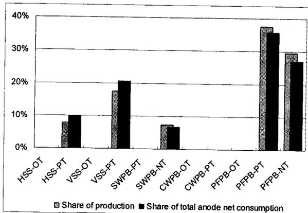
Figure 6: Share of production and total anode consumption of different technical categories of Al electrolysis cells in 2010 according to case study 2.
