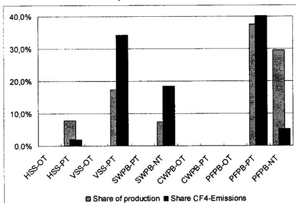
Figure 9: Share of production and total CF<sub>4</sub> emissions from smelters of different technical categories in 2010 according to case study 2.
