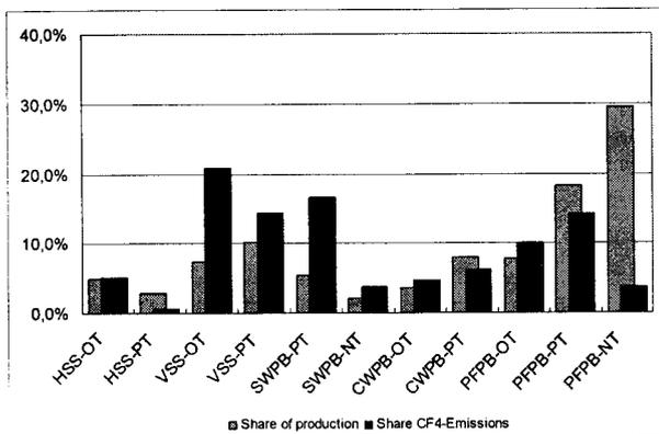
Figure 8: Share of production and total CF<sub>4</sub> emissions of different smelter categories in 2010 according to case study 1.
