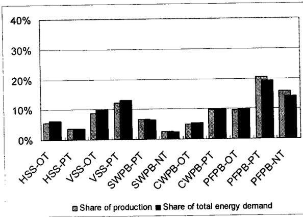
Figure 1: Share of production and total energy requirement for different technical categories of Al electrolyses cells in 1997.
