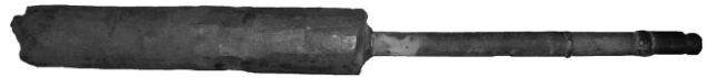
Fig. 3. Electrode prepared for ESR by forging and welded to power connection (stub).
