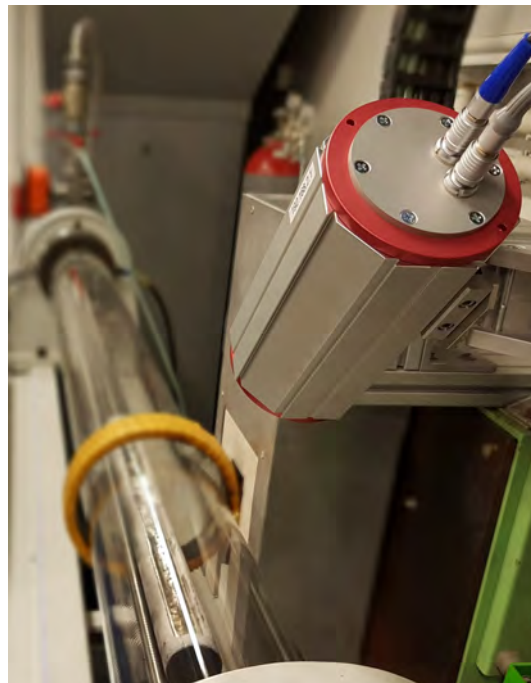
Figure 2. Infrared camera setup focusing on the molten zone region below the induction coil.
