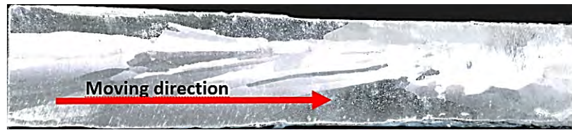
Figure 12. Macrograph of the longitudinal section, in the position at the middle of the bar (done using Barker's reagent for 30 s at room temperature).
