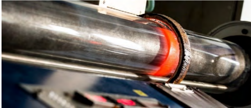
Figure 1. Horizontal zone refining equipment with a single induction heater (photo by Martin Braun).
