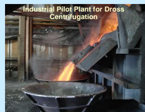
Centrifugation of as-produced aluminium drosses in industrial pilot scale (Centrifuge T3, Italy)
