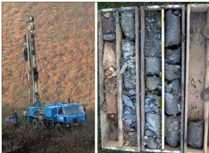
Fig. 1: Drilling equipment (left) and received drilling cores (right)
