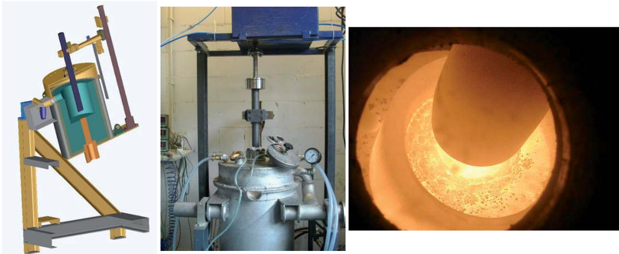
Figure 3: Schematic drawing and photograph of the EAF used. On the right picture of the reaction zone during operation (the graphite crucible is seen in the bottom while the hollow electrode tip is directly above it). No liquid melt formation is observed.
