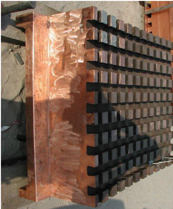
A- New Hatch Coolers
