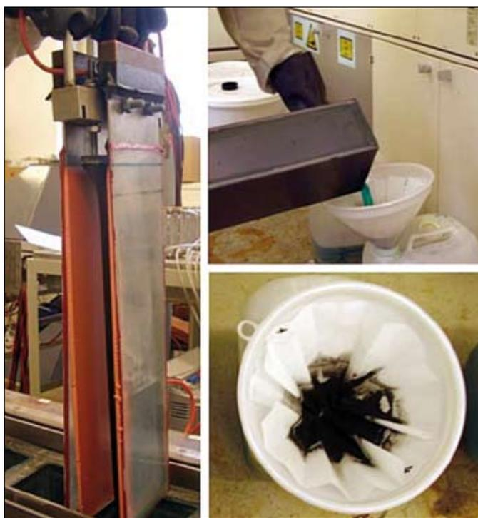
Fig. 1: Removing of electrodes, filtering of electrolyte and remaining anode sludge after electrolysis
