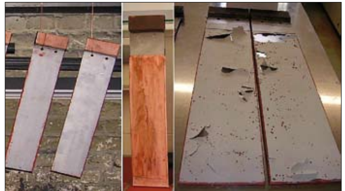
Fig. 4: Cathode sheets before (front side) and after electrolysis (front with approx. 1000 g Cu deposition and back)
