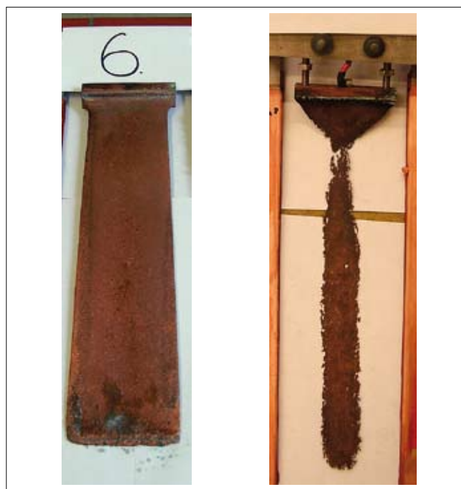
Fig. 1: Left: regularly dissolved anode at 409 A/m 2 ; right: strongly dissolved anode at 409 A/cm 2
