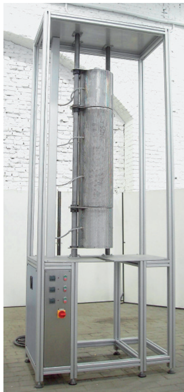
Fig. 9a: Furnace with three different heating zones
