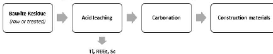
Figure 4: A near zero waste valorisation vision for bauxite residue after smelting through experimental results for cement industry
