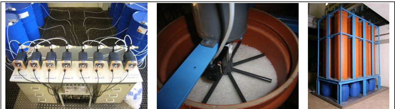
Figure 6: Experimental set-up: pumps with control system and storage drums (left), sprinkler system (middle) and the IME-8-column set-up (right)
