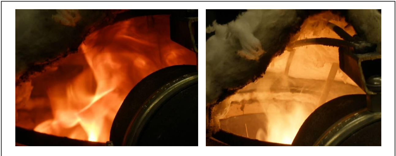
Figure 3: Off-gas from the direct melting process at the beginning (left) and at the end (right) of the experiment
