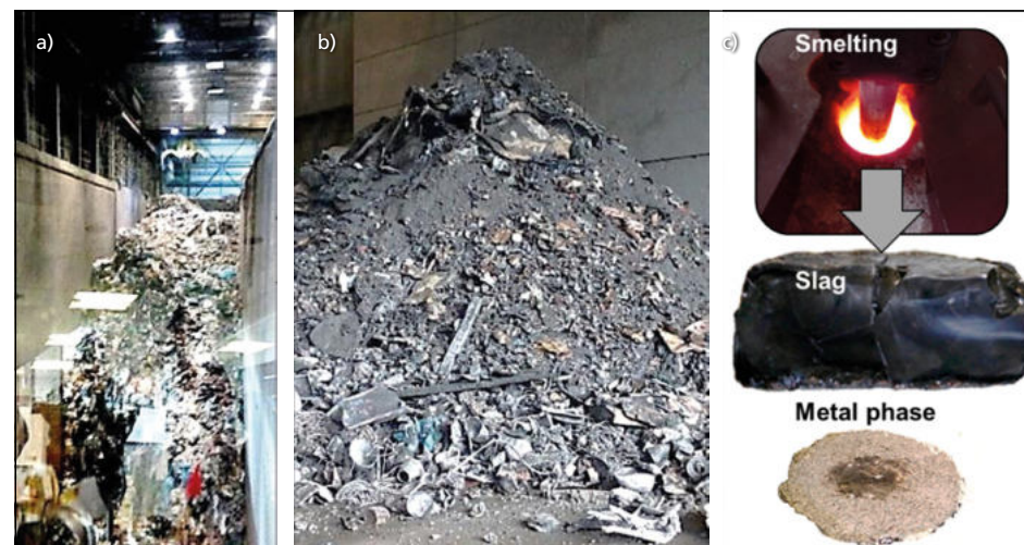
Figure 13: Municipal solid waste (a) before incineration, (b) bottom ashes remaining after incineration (IBA) and (c) vitrified IBA and the recovered metal phase
