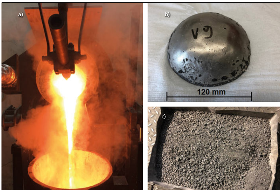
Figure 11: Emptying SAF after (a) slag cleaning, (b) metal phase and (c) slag phase
