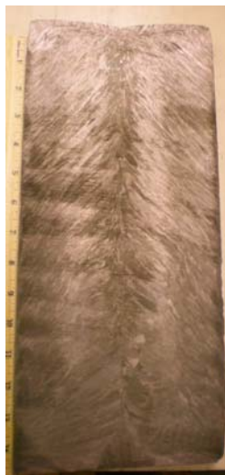
Figure 5: Macrostructure from ingot 7, higher pressure and Si 3 N 4 .
