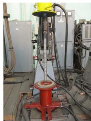
Figure 4: The chamber electroslag furnace A-550 (724 kW) The remelting was conducted under a flux of pure CaF 2 (TU 6-09-5335-88). The flux was melted directly in the crucible, using the technology of "solid" start. The starting mixture was prepared of titanium chips and the operating flux. The electrical parameters of the refining maintained at U = 36.0 V and I = 2.0-2.5 kA, providing a good surface quality of the remelted ingots (Figure 5).
