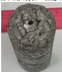
Figure 3: Pressed block of titanium sponge with carbon powder filled into the drilled axial hole
