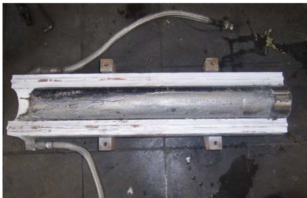
Figure 6: VIM-cast TiAl electrode ( \varnothing 105 mm, L 750 mm, mass approx. 25 kg)
