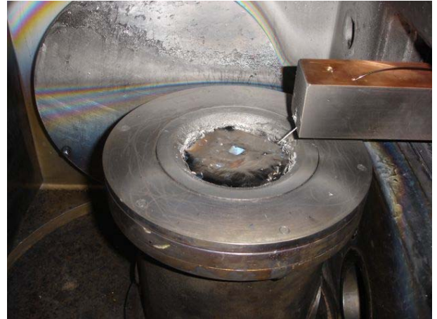
Figure 11: loaded water-cooled crucible and optical fibre measurement set-up
