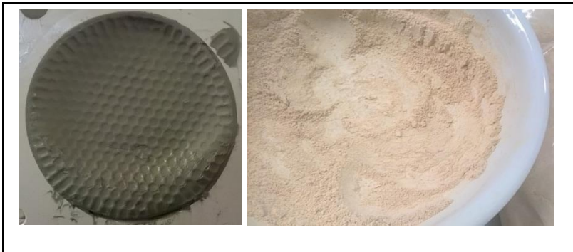
Figure 3: Filter cake after fuming, leaching, neutralisation, filtration (Left) and produced REE-carbonate (right)
