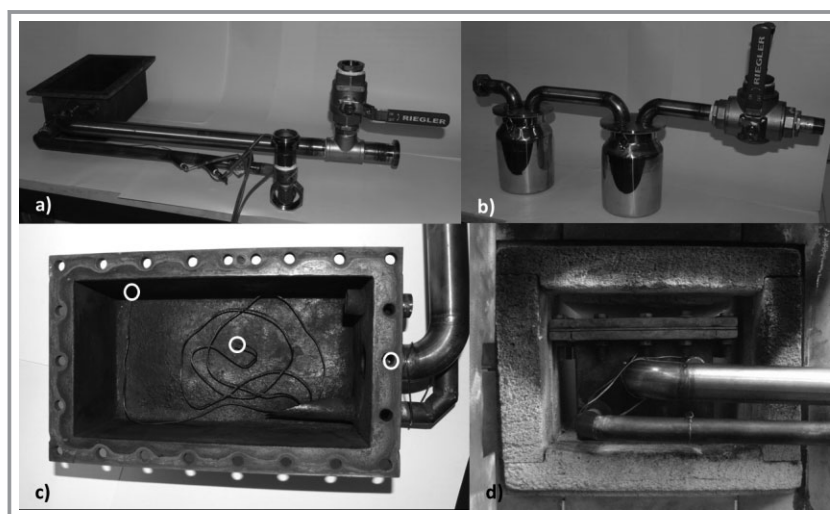
Figure 6. Equipment and setup for pyrolysis experiment: a) locked pyrolysis batch reactor, b) condensate bins, c) open pyrolysis reactor with measuring points for temperature, d) pyrolysis reactor in the furnace.
