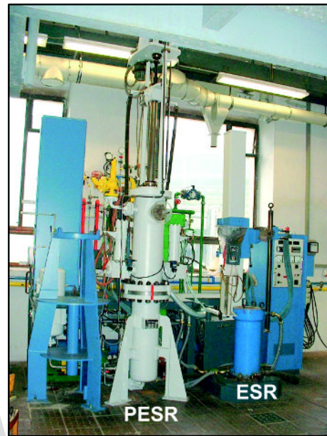
Figure 10. PESR/ESR pilot scale furnace at IME Aachen.
