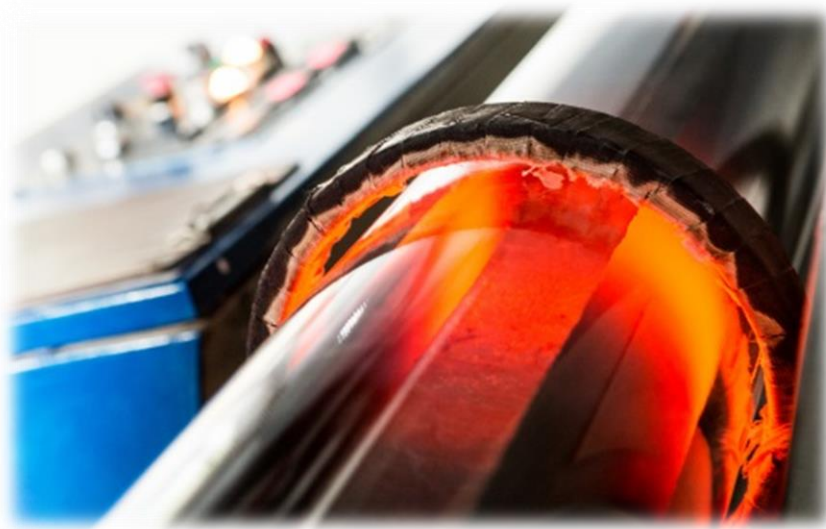
Figure 2: Zone melting equipment at IME and its moving glowing hot zone
