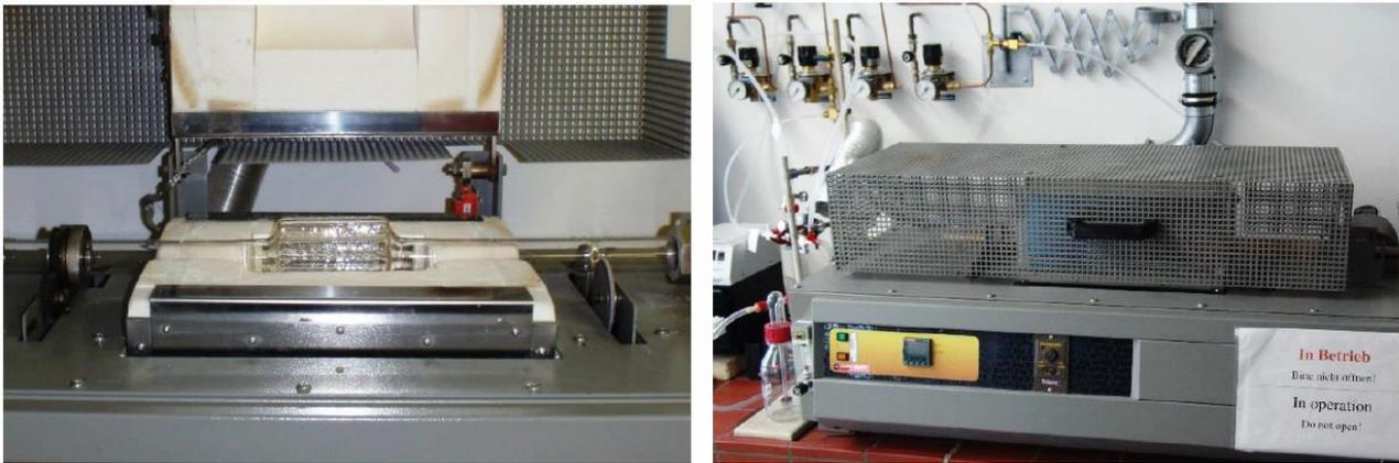
Figure 6: Carbolite rotary furnace used for thermal decomposition of lead citrate
