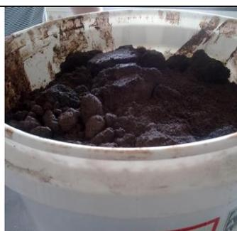
Figure 1: Lead Paste Scrap
