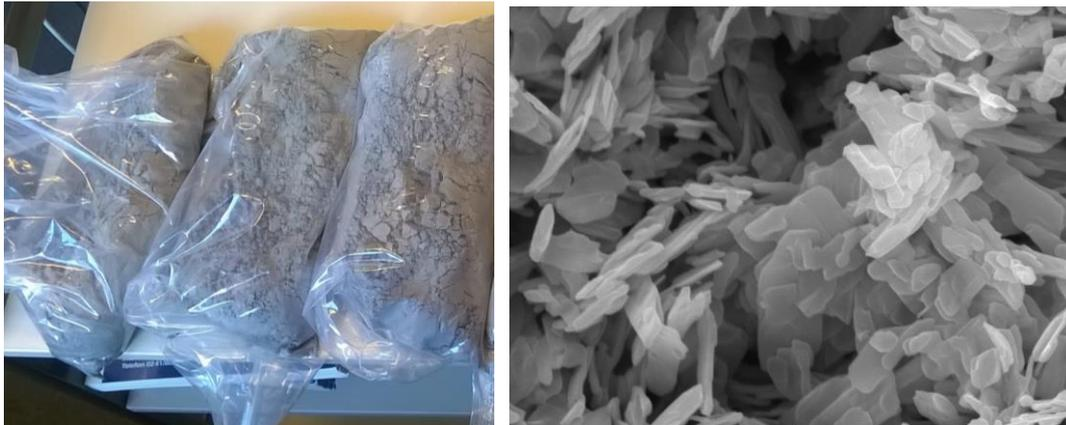
Figure 4: Produced lead citrate in 200 L reactor with a typical SEM image of a filter cake
