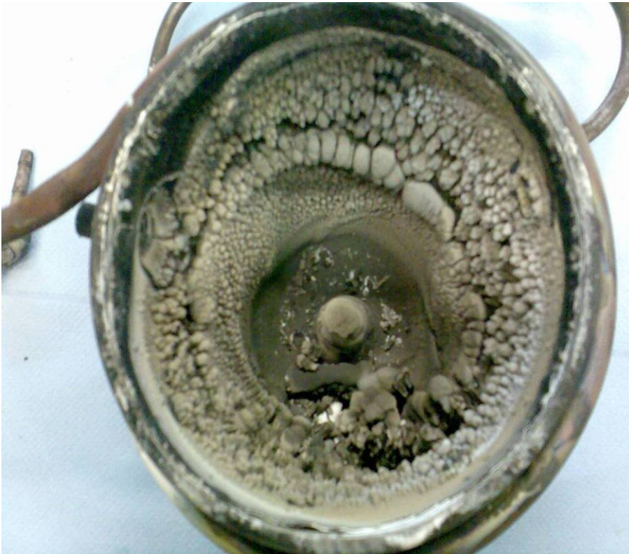
Condensate inside the chamber
