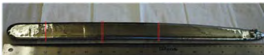
Figure 7. Effect of the mass transport into the bar as the molten zone moves across the bar for a system with a melt density higher than the solid, e.g., germanium [40].
