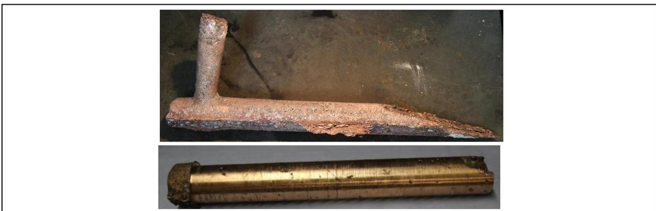
Figure 6: Metal product of ATR in-line casting untreated and prepared for VAR process
