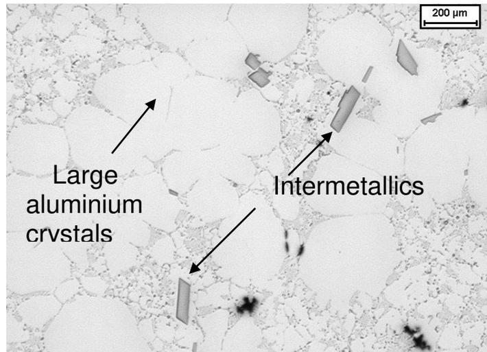
*Figure 3, sample taken from a typical experiment in the MAP project showing the existence of intermetallics separated from the aluminium primary crystals*
