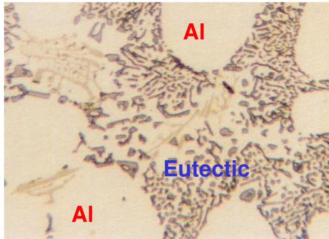
*Figure 2, Typical Aluminium structure after casting clearly showing the aluminium crystals (earliest formed material) and the region where the combined formation of Intermetallics and aluminium took place (denoted with eutectic)*
