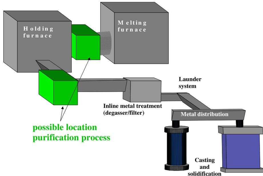
Figure 4, Schematic representation of the application of the MAP process inside the existing production process of ingot and billet casting
