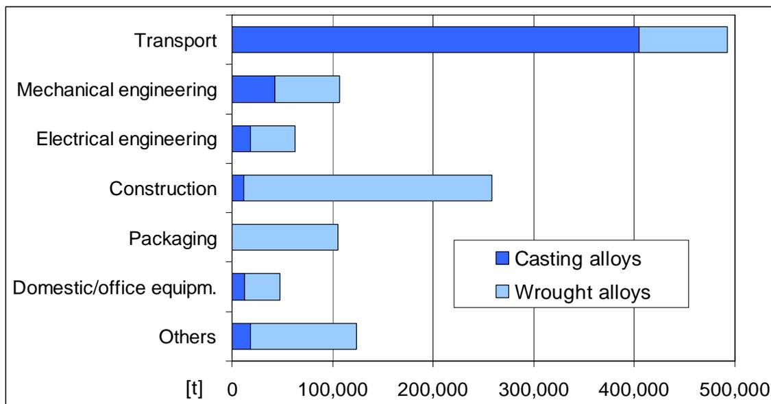
Figure 3: Use of aluminium casting and - wrought alloys 1997 [ 2 ]
