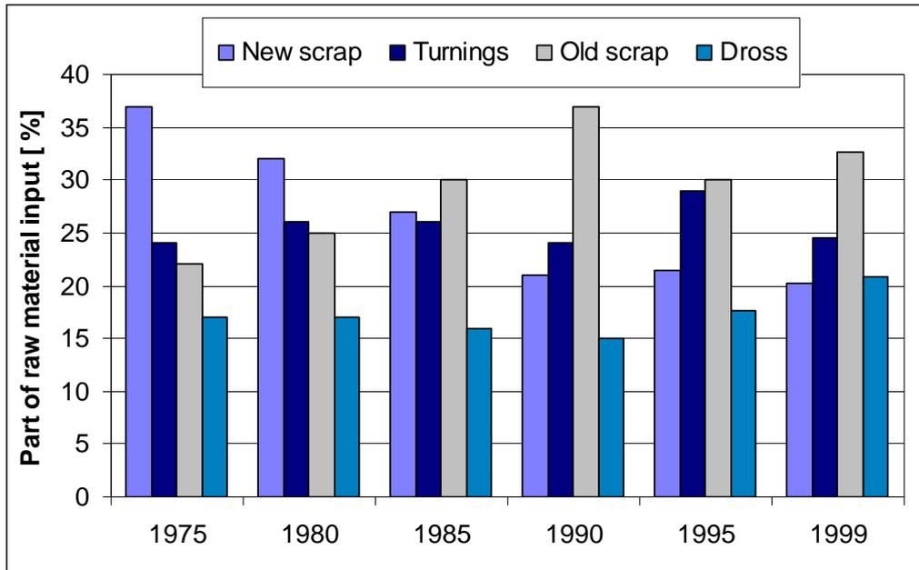
Figure 11: Development of the scrap supply of the German secondary aluminium smelters from 1975 to 1999 [7]
