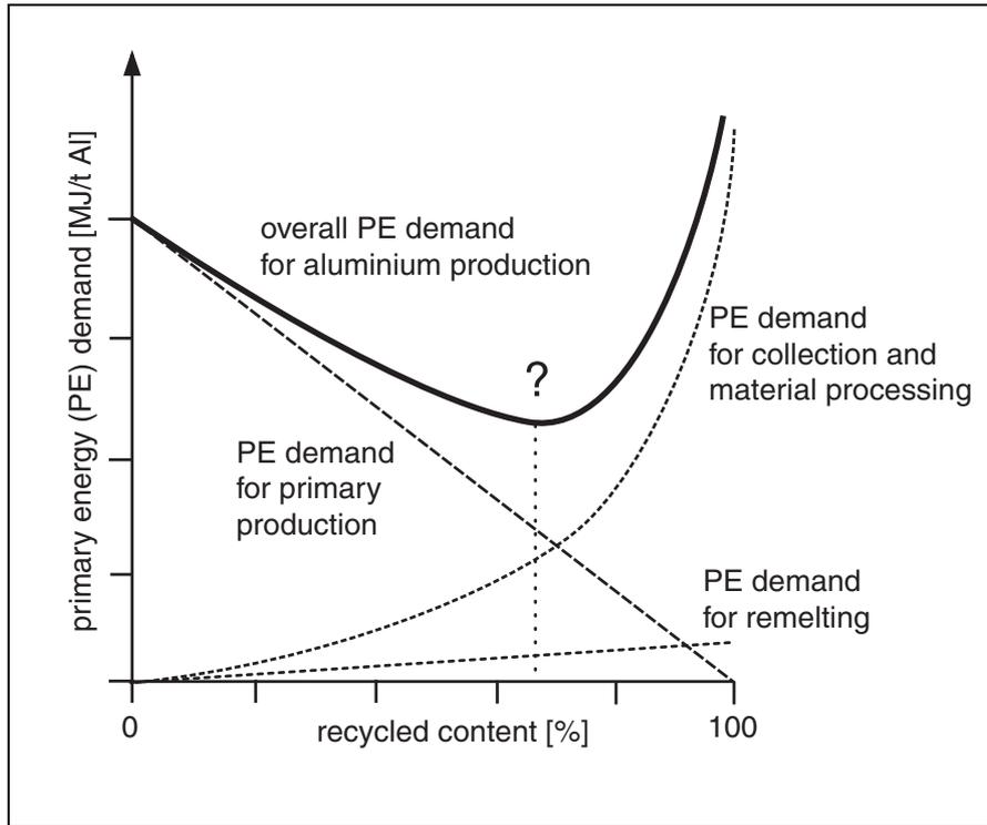
Figure 14: Qualitative determination of an optimal recycling ratio regarding the primary energy expenditure
