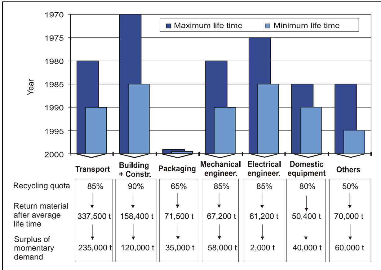
Figure 6: Recycling quotas and return quantities resulting from different lifetimes for different applications under the assumption of complete collection
