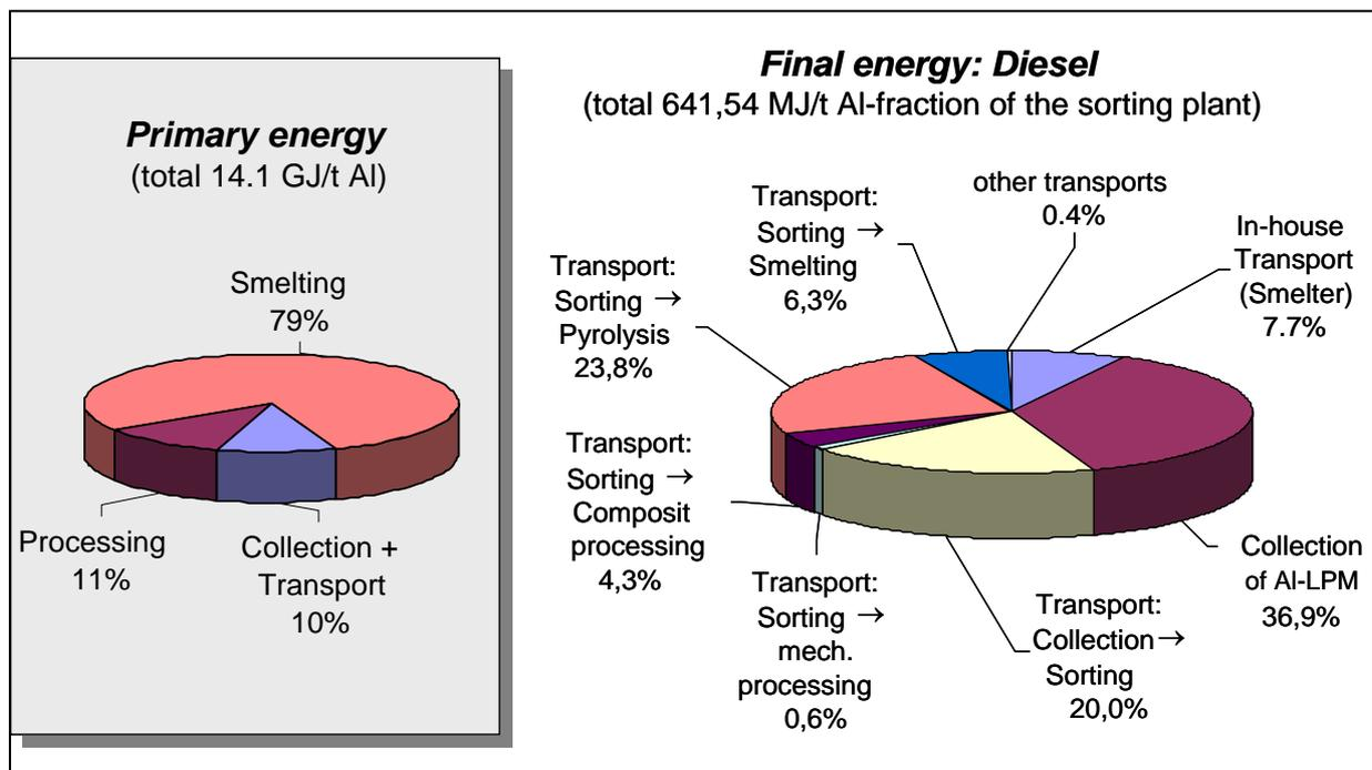
Figure 18: Classification of the primary and final energy consumption for the packaging recycling by the example of Diesel fuel [ 10 ]
