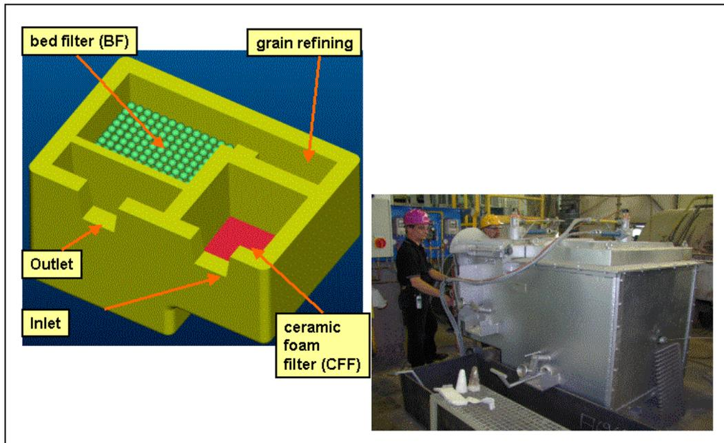
Figure 14: In line aluminium melt treatment: Hydro (VAW)-Filter
