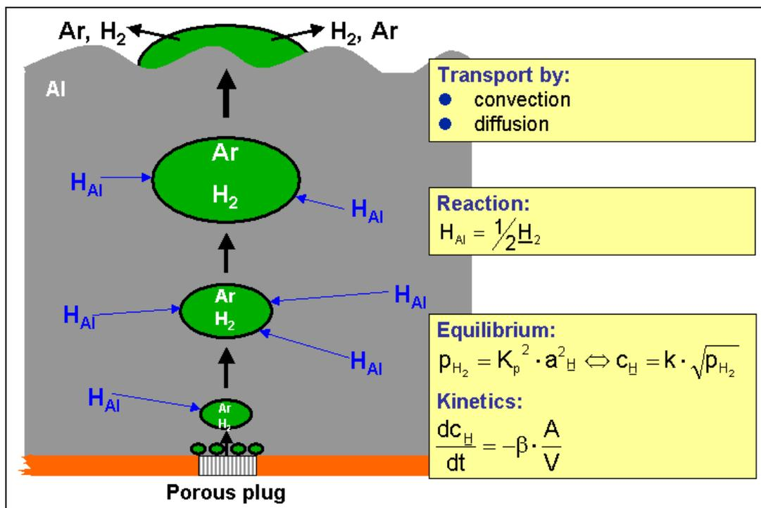
Figure 6: Principle of gas purging
