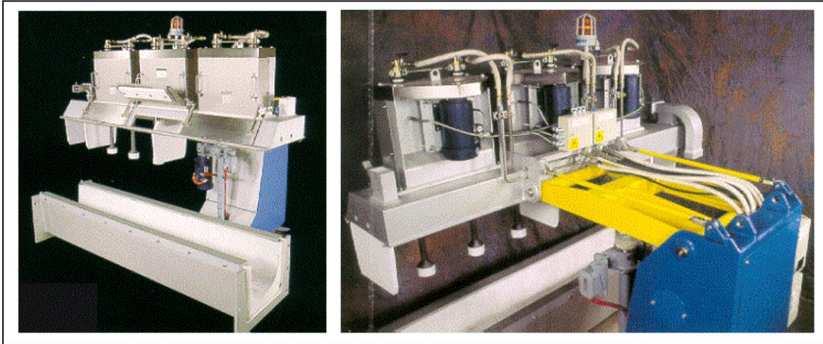
Figure 10: In line aluminium gas purging: Alcan Compact Degasser
