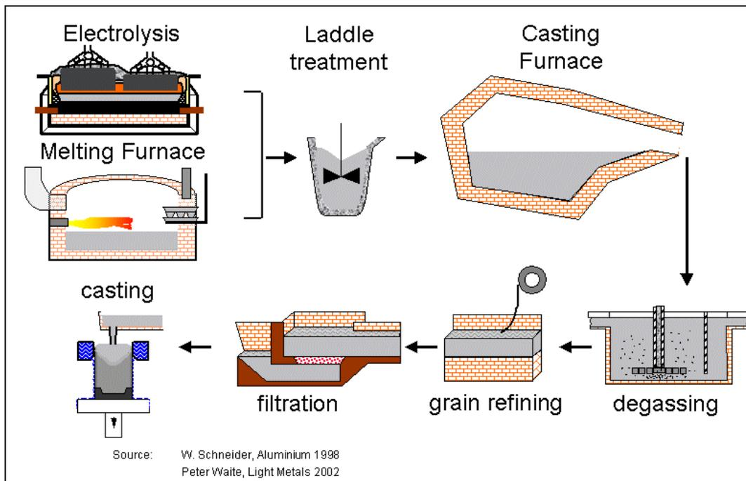
Figure 5: Processing of molten aluminium
