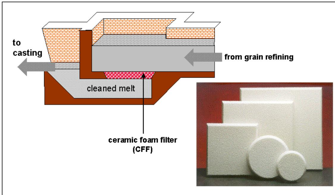
Figure 13: Technology of aluminium melt filtration
