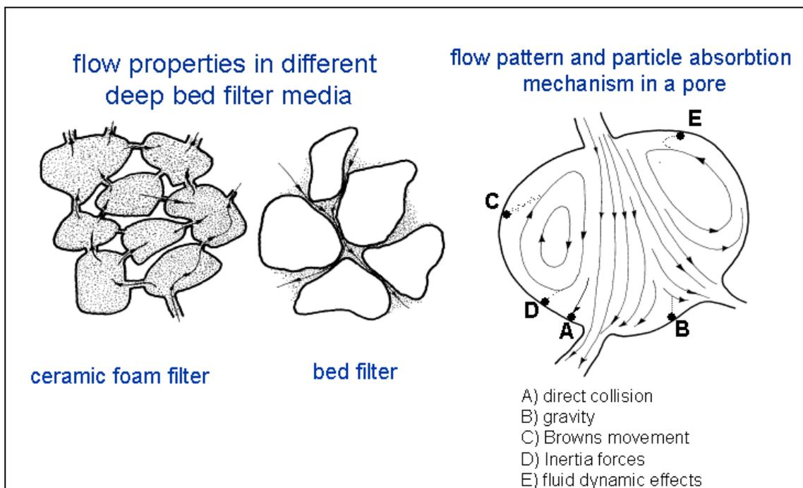
Figure 11: Principles of melt filtration
