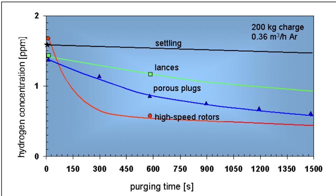
Figure 8: Efficiency of gas purging methods
