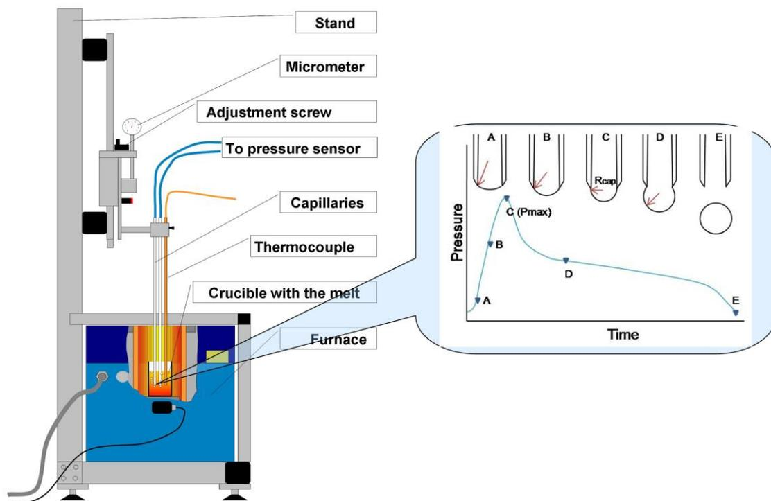
Fig. 8: Instrument and principle of surface tension measurement based on max. bubble pressure method
