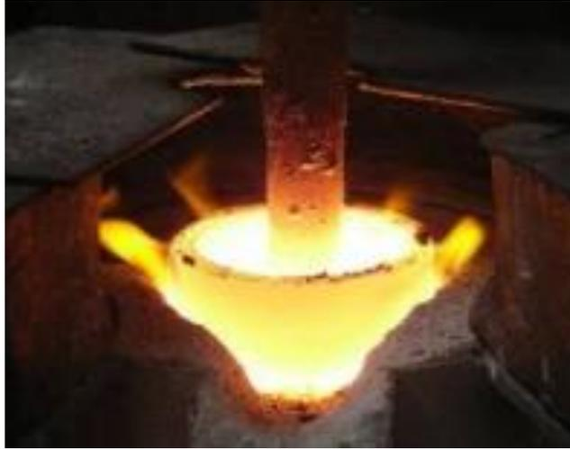
Figure 4: Lab-Scale battery recycling in an EAF at the IME
