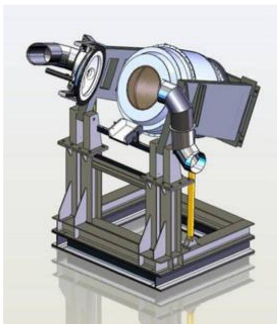
Fig. 10: Large scale TBRC for WEEE-scrap recycling
