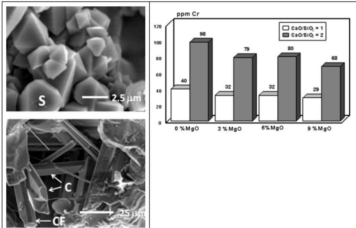
Fig. 2: SEM micrographs of the crystalline phases of the slag with 3 % MgO and  $\text{CaO}/\text{SiO}_2 = 2$ . CF:  $\text{Ca}_5(\text{CrO}_4)_3\text{F}$ . C: cuspidine ( $\text{Ca}_4\text{Si}_2\text{O}_7\text{F}_2$ ). S:  $\text{MgCr}_2\text{O}_4$  spinel (left side) and the effect of the  $\text{CaO}/\text{SiO}_2$  ratio and MgO content on the leaching behaviour of Cr (right side).
