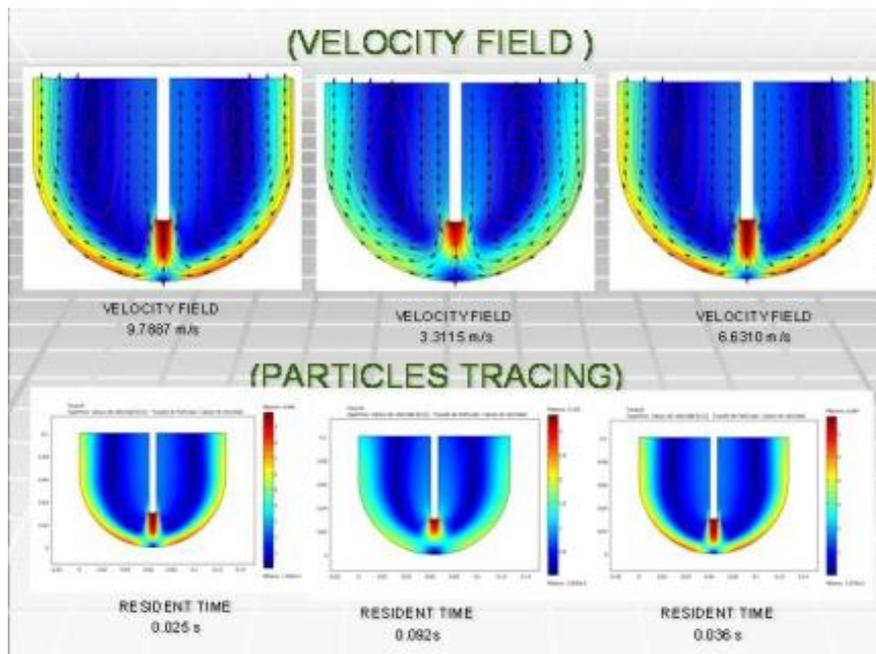
Fig. 1: Simulation of velocity fields and particle tracing of powder injection into a molten lead bath
