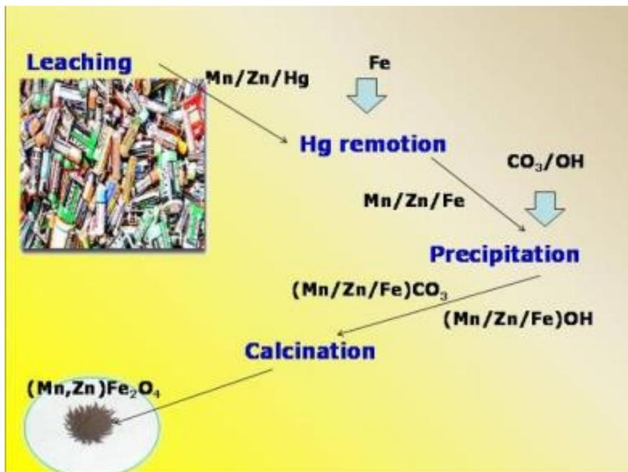
Fig. 6: Hydrometallurgical battery recycling by obtaining Mn/Zn ferrites
