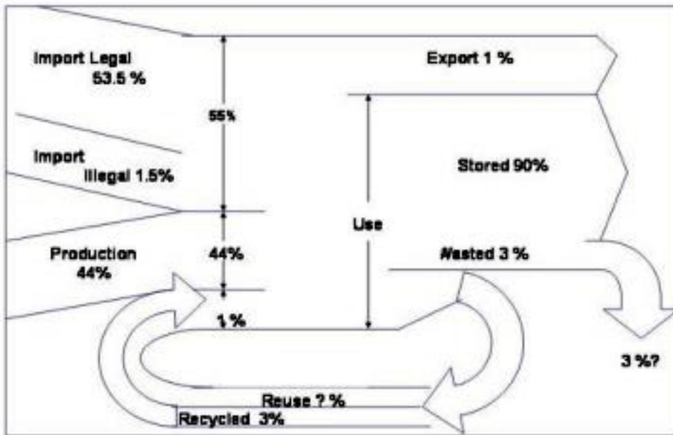
Fig. 9: Materials balance of electronic goods in México
